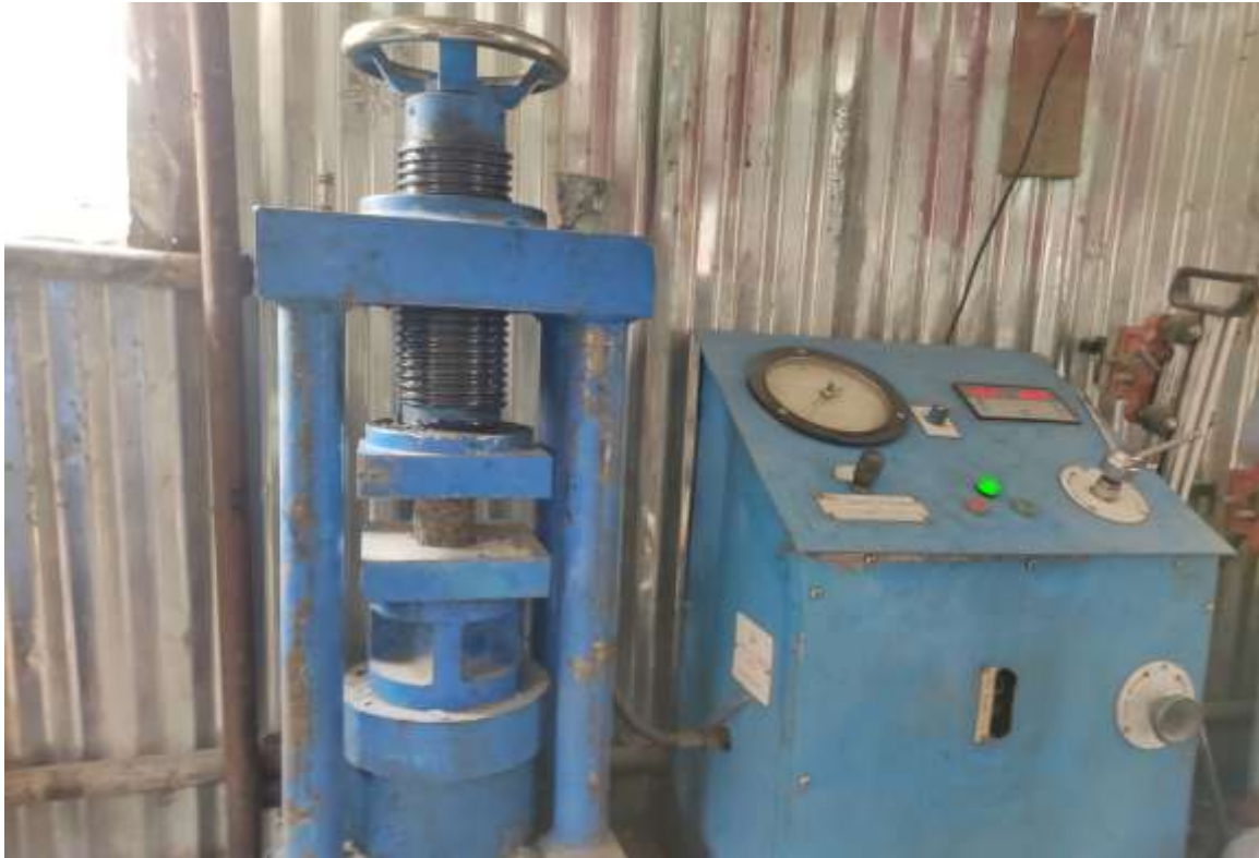
Figure 25: Compressive strength test of shotcrete core
